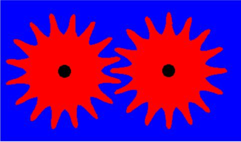
What you can see includes this: As a tooth near the centre of the picture moves up or down it will come into contact with a tooth from the other wheel.
