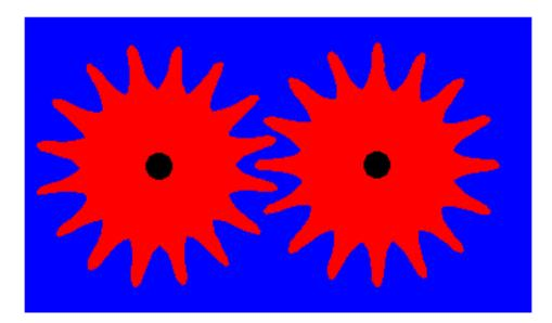
As a tooth near the centre of the picture moves up or down it will come into contact with a tooth from the other wheel.
