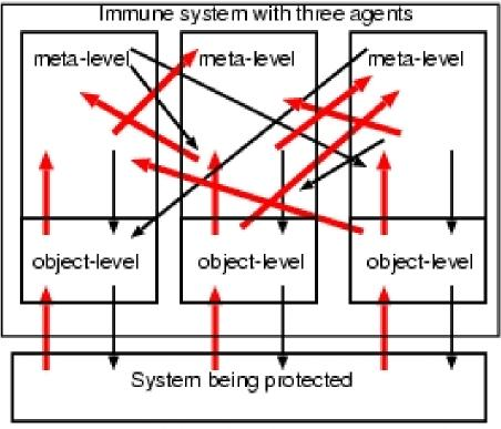
red thick upward arrows: sensing black thin downward arrows: acting (Not all possible arrows shown)
