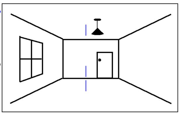
Some pairs of parallel edges in the scene are represented by parallel picture lines, others by converging picture lines.
