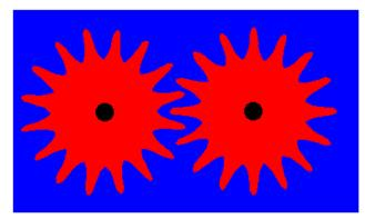
In this case, using the constraints of the theory you can work out that if the left wheel rotates clockwise the right wheel must rotate anti-clockwise – and *vice versa*. (How?)
