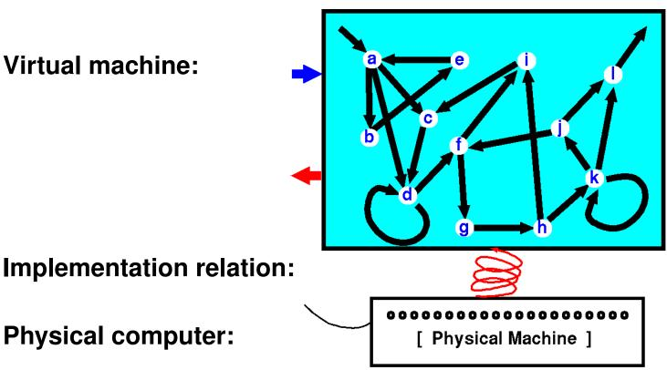
The virtual machine that runs on the physical machine has a finite set of possible states (a, b, c, etc.) and it can switch between them depending on what inputs it gets, and at each switch it may also produce some output.
