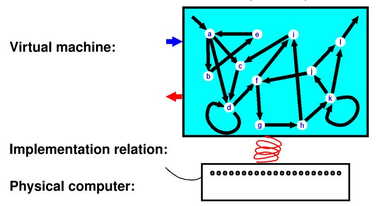
The virtual machine that runs on the physical machine has a finite set of possible states (a, b, c, etc.) and it can switch between them depending on what inputs it gets, and at each switch it may also produce some output. This is a fairly powerful model of computation: but it is not general enough.
