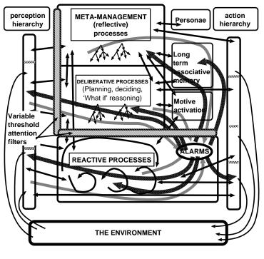
Arrows represent information flow (including control signals). The alarm mechanisms receive information from many sources and using fast (but possibly stupid) pattern recognition mechanisms decide whether to send out high priority global signals to cause freezing, re-direction, or modulation of behaviours.
