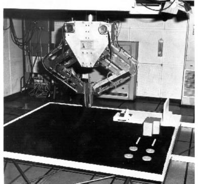
E.g. Freddy could not simultaneously see and act: partly because visual processing was extremely slow. Imagine using a computer with 128Kbytes RAM for a robot now.
