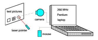
Fig. 6.1. The simulation system
