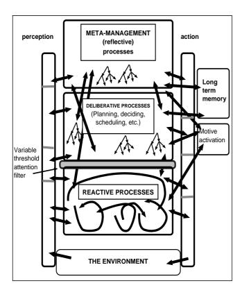
Figure 5: Towards a human-like reflective architecture: the previous system with mechanisms able to monitor, categorise, evaluate and modify processes in other systems.
