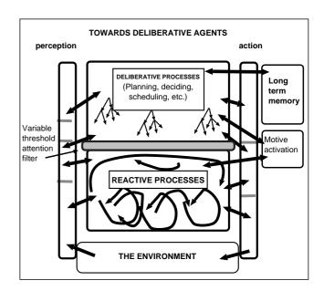
Figure 3: A hybrid system combining reactive and deliberative mechanisms.
