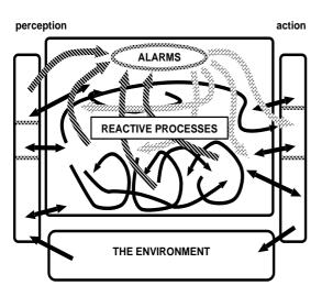
Fig. 4. A reactive system with global alarms. When reactive systems are so complex and sophisticated that they can introduce significant delays between sensing and acting, it may be useful to have a more 'stupid' pattern-directed alarm system, with inputs from everywhere and outputs going to all parts of the system, which can take control when emergencies or urgent opportunities are detected.
