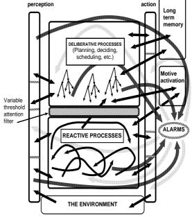
Fig. 5. A hybrid architecture with global alarms. Reactive and deliberative mechanisms may sometimes be dominated by control signals from a global alarm system.
